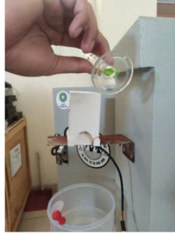
Fig. 12. Process rainfall sensor calibration.
