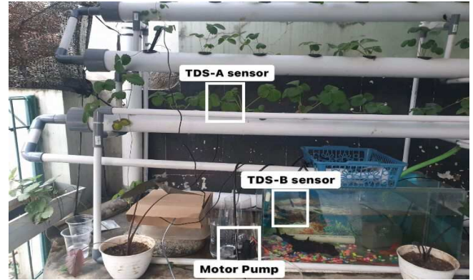
Fig. 6. Implementation aquaponic DFT.
