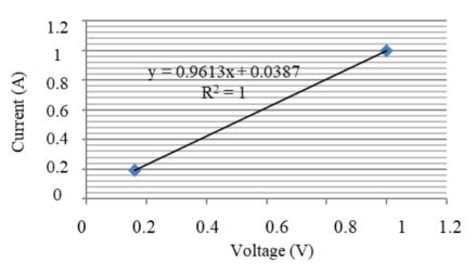
FIGURE 4. The Relationship of Voltage (V) and Current (I) in a Parallel Circuit
