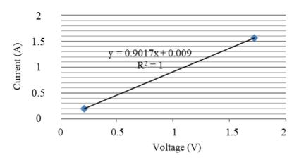
FIGURE 3. The Relationship of Voltage (V) and Electric Current (I) in a Series Circuit
