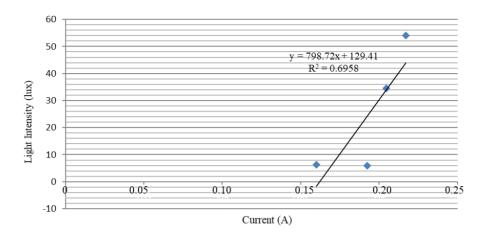
FIGURE 5. Relation of Electric Current (I) to Light Intensity (I)
