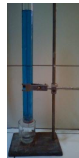
GAMBAR 2. Uji Permeabilitas Filter
