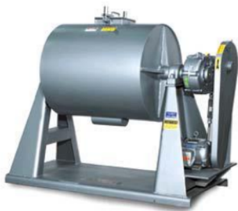
Figure 1. The schematic diagram of the ball milling reactor for the fabrication of duck eggshell powders (Abdullah, 2008).
