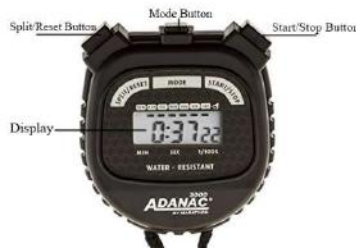
Gambar 5. Bagian-Bagian Stopwatch Digital
