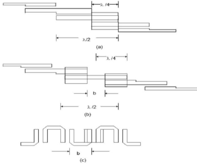
Fig. 1. Parallel-Coupled Line Transformation into Hairpin Filter [8]
