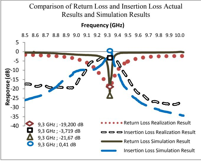
Fig. 6. Comparison of Return Loss and Insertion Loss Actual Results and Simulation Results
