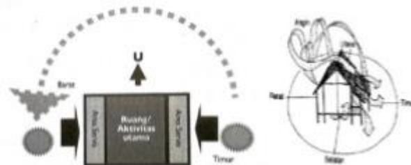
Figure 4. Building orientation based on the direction of the sun movement and the wind
